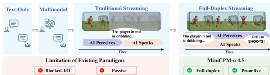
Figure 3: From turn-based interaction to full-duplex streaming. Existing interaction paradigms separate perception and response as alternating phases, leading to blocked information flow and passive behavior. In contrast, MiniCPM-o 4.5 continuously perceives incoming multimodal streams while speaking, allowing the model to update its response in real time and act proactively.
