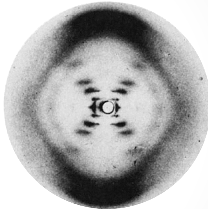
The key X-ray photograph involved in the elucidation of the DNA structure. (Rosalind Franklin, winter of 1952–1953)
