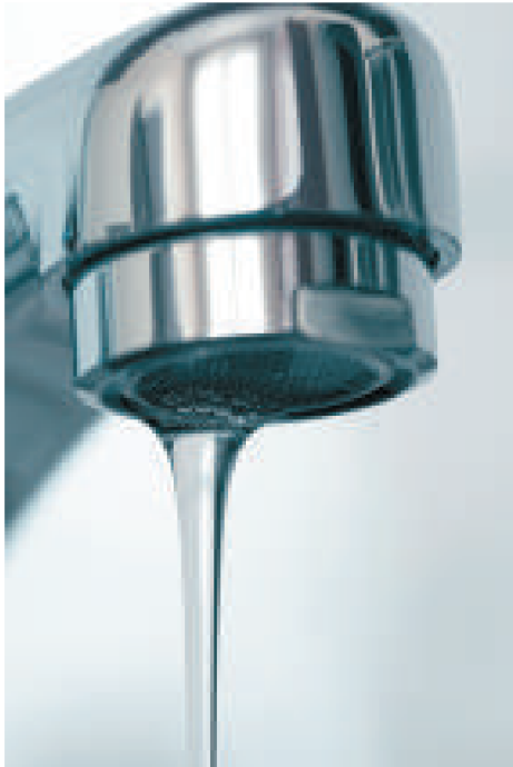
(a) Low speed: laminar flow
